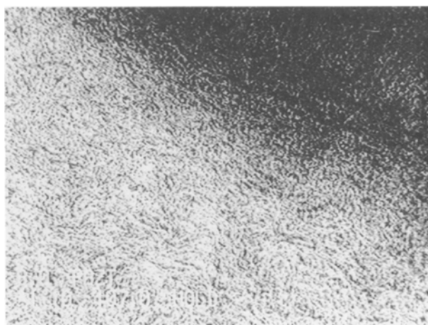
Figure 4 Growth of the red crystal solvate out of a nematic homogeneous solution of PBZT (8%) in PPA at 160 °C; \times 320 .
